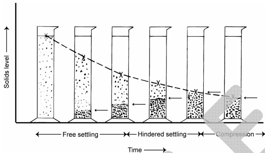
**Figure 2-3 – Settling of agglomerated particles. (courtesy of Nalco)**
